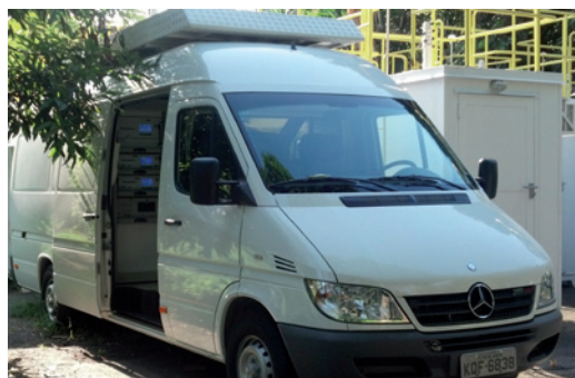
Example of mobile air quality monitoring station with rack version 2M series analyzers.
